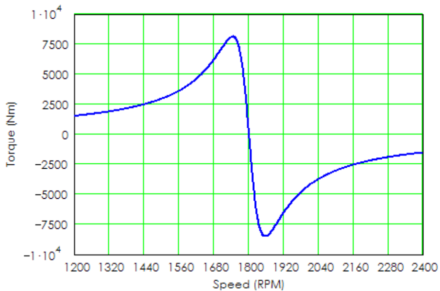
Figure 4: Torque vs. speed characteristics for a squirrel cage induction generator.
